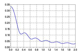
For  $w \to 0$  we obtain the value 1/3 corresponding to the piecewise constant case  $|\rho| = \lfloor 1/2 - 1 \rfloor / (1/2 + 1) \rfloor$ . As the transition becomes more gradual, the reflection coefficient drops quite rapidly. This is a general result; smooth transitions produce very small reflected fields. This idea leads to a simple
