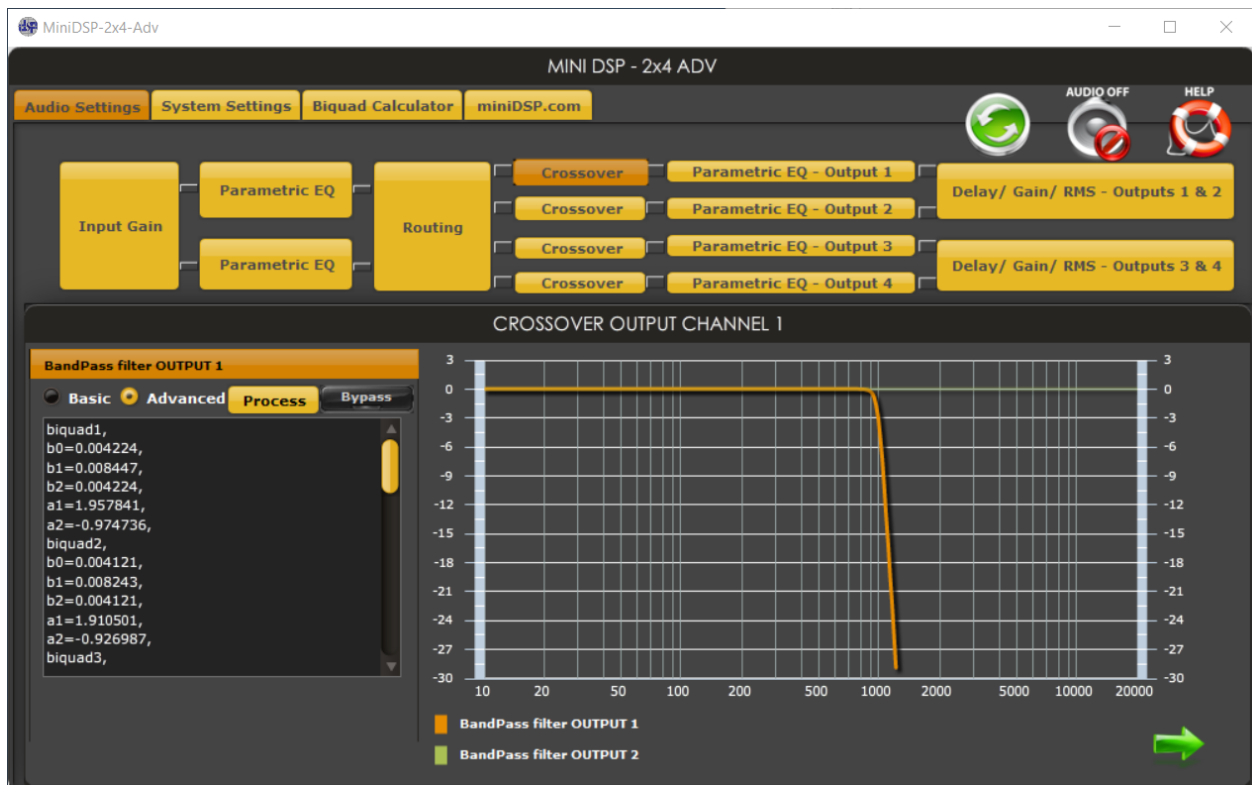
Fig. 3: MiniDSP plugin. Sixteenth-order Butterworth lowpass filter entered as cascade of eight biquads.
