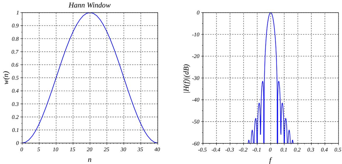
Fig. 3: (Left) Hann window for  $M = 40$ . (Right) Magnitude frequency response (normalized).
