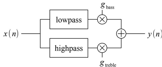
Fig. 13: Two-band equalizer.
