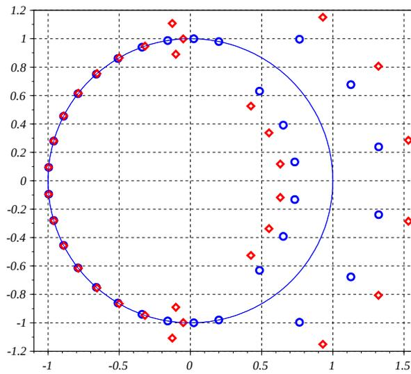
Fig. 12: Lowpass filter  $z$ -plane zeros with (circles) rectangular window and (diamonds) Hamming window.
