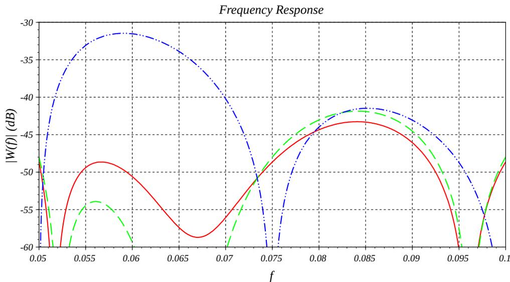
Fig. 5: Response of  $M=40$  Hann (blue dot-dash), Hamming (green dashed), and modified Hamming (solid red).
