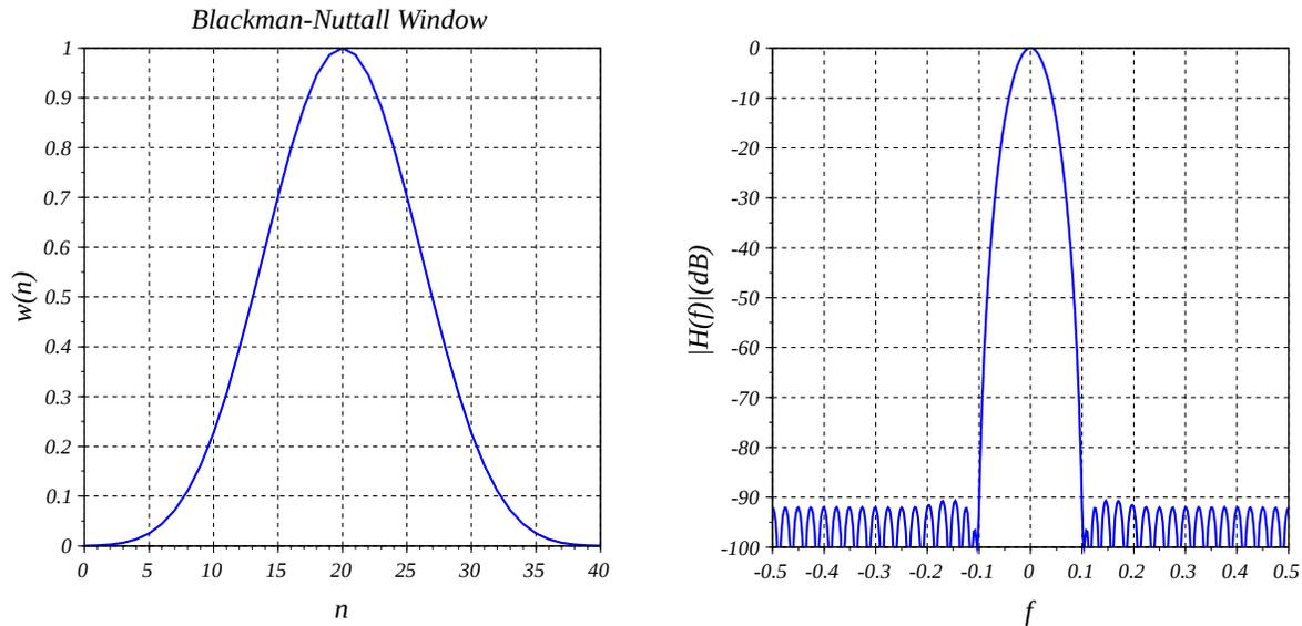
Fig. 6: (Left) Blackman-Nuttall Window for  $M = 40$ . (Right) Magnitude frequency response (normalized).
