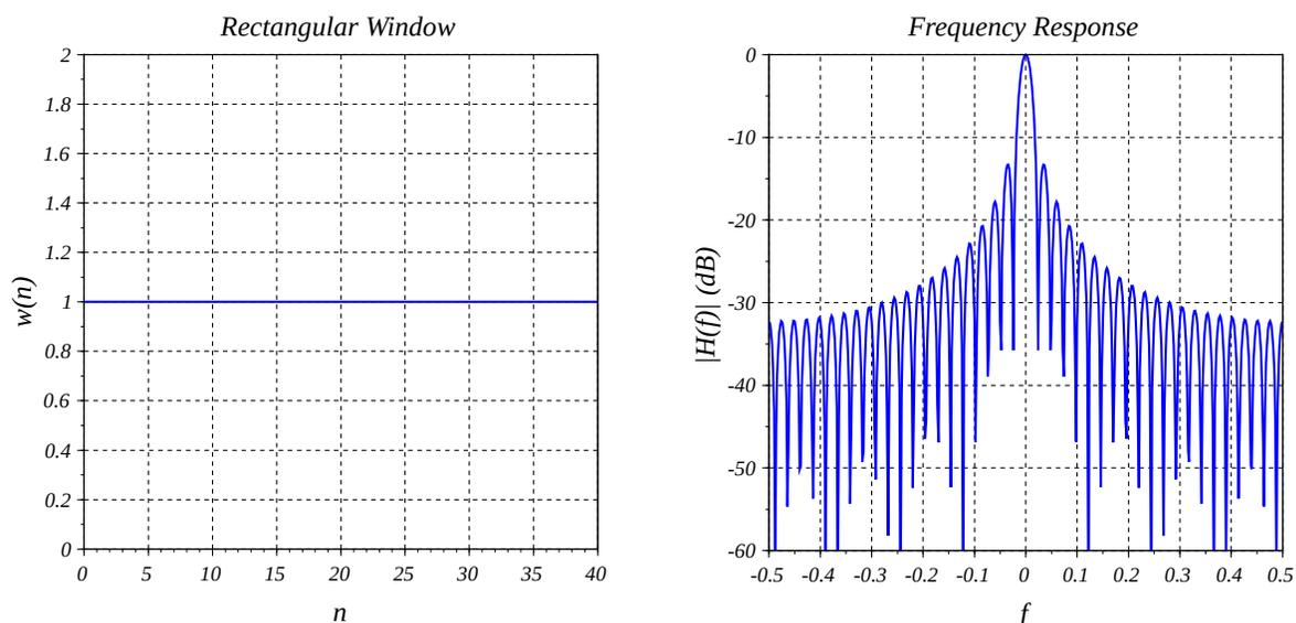
Fig. 1: (Left) rectangular window for  $M = 40$ . (Right) magnitude frequency response (normalized).
