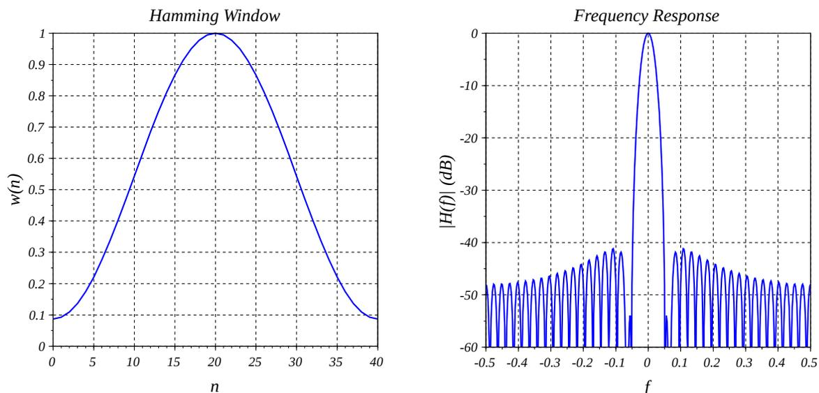
Fig. 4: (Left) Hamming window for  $M = 40$ . (Right) Magnitude frequency response (normalized).
