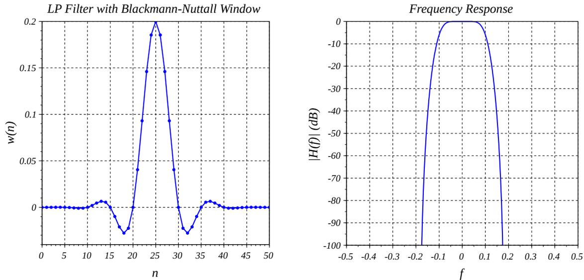
Fig. 10: Lowpass filter with Blackman-Nuttall window.
