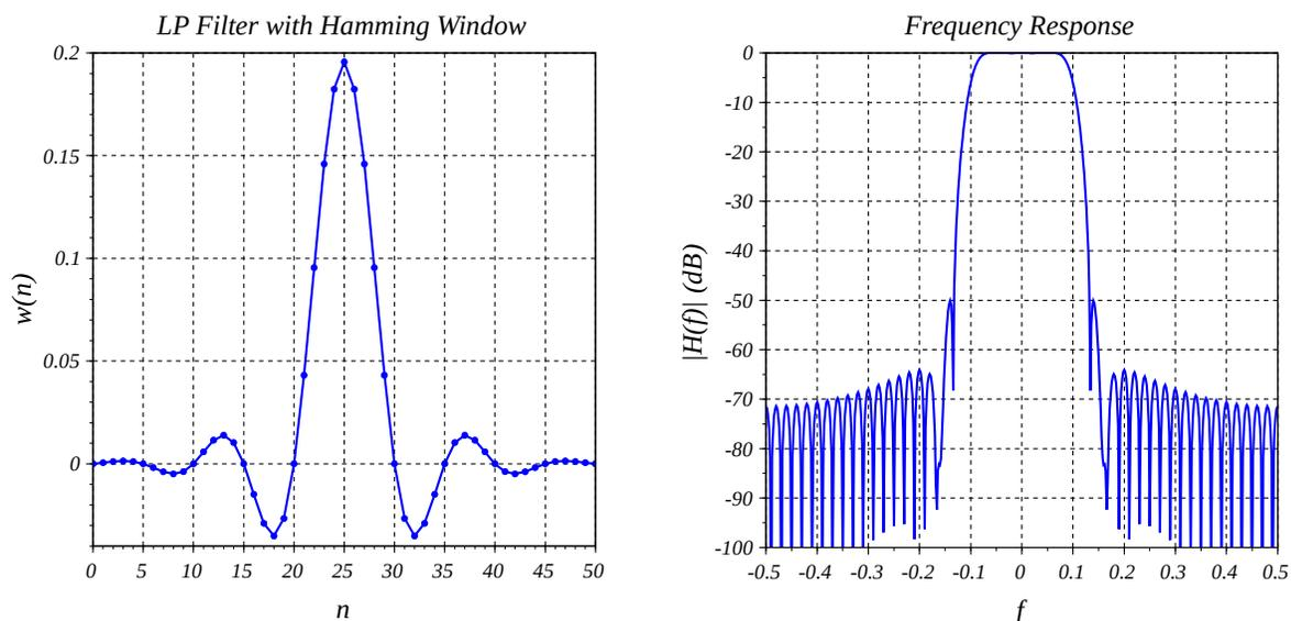
Fig. 9: Lowpass filter with Hamming window.
