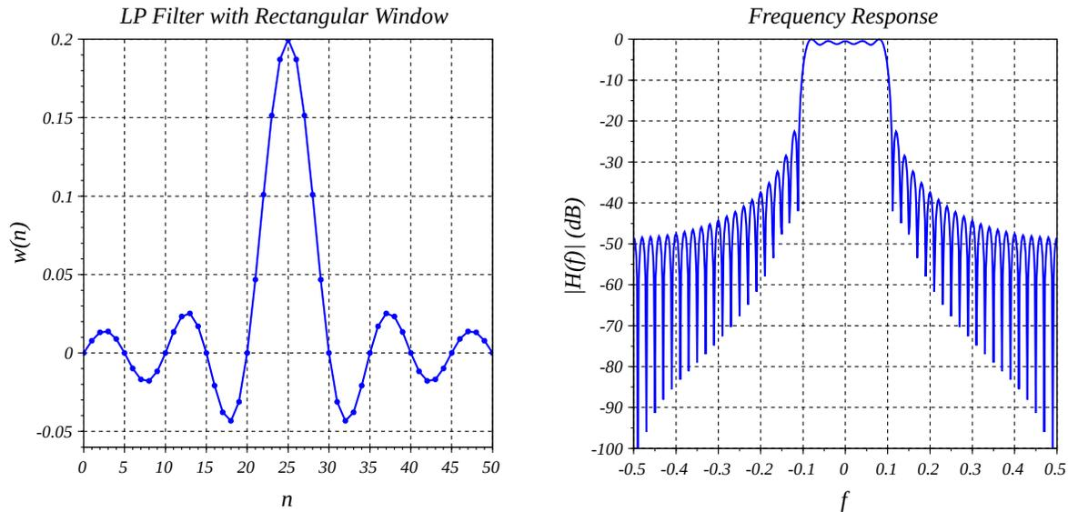
Fig. 8: Lowpass filter with rectangular window. (Normalized to 0 dB peak frequency response.)
