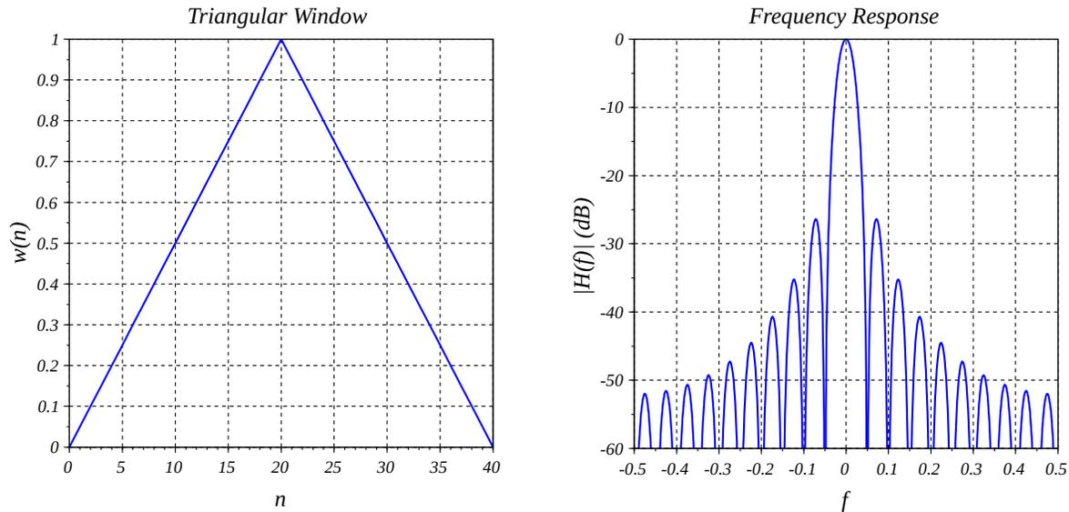
Fig. 2: (Left) Triangular window for  $M = 40$ . (Right) Magnitude frequency response (normalized).
