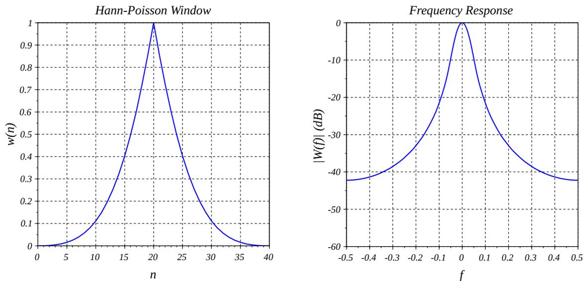
Fig. 7: (Left) Hann-Poisson Window for  $M = 40$ . (Right) Magnitude frequency response (normalized). This window has the property that its frequency response decreases monotonically, so there are “no sidelobes.”
