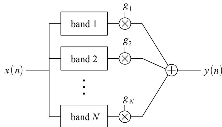
Fig. 14:  $N$ -band equalizer.
