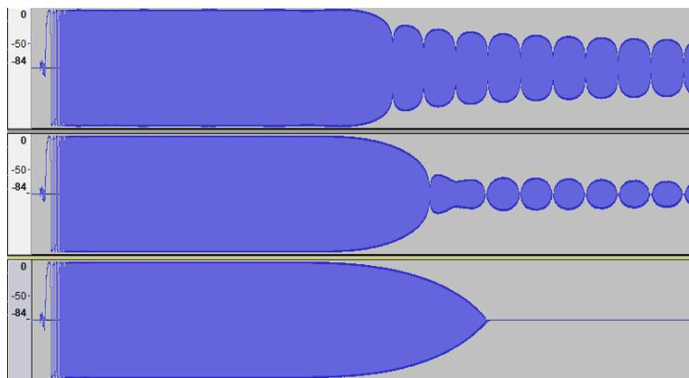
Fig. 11: Lowpass-filtered chirp signal using (top) rectangular, (middle) Hamming, and (bottom) Blackman-Nuttall windows. Amplitudes are in dB ranging from 0 to  $-84$  dB. (Audacity screenshot.)
