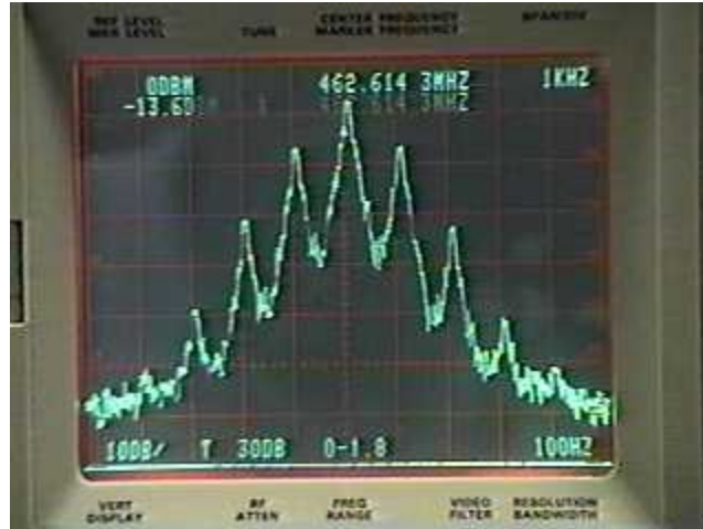
Figure 20.4: Spectrum of a 462-MHz FM radio transmission with 1kHz modulation.
