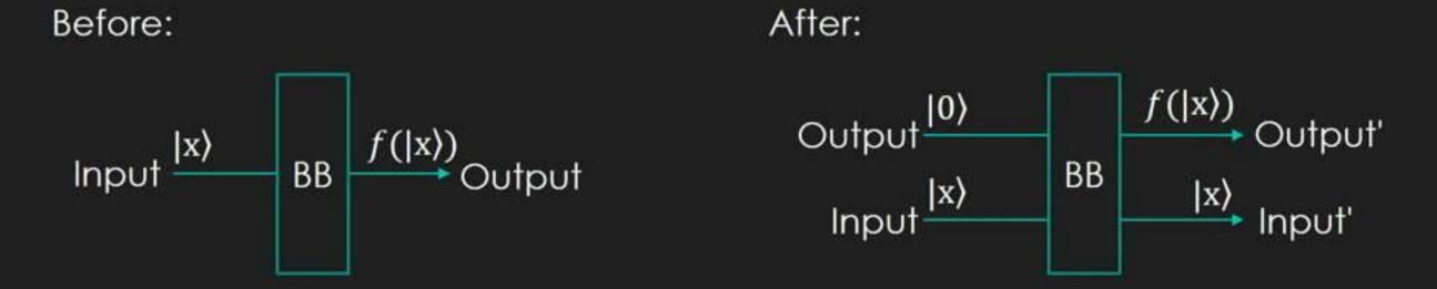
The black box leaves the input qbit unchanged, writing function output to output qbit
