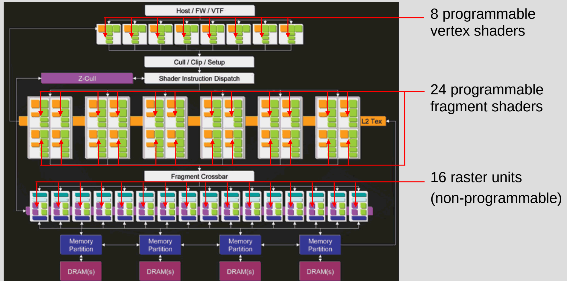
GeForce 7800 GTX block diagram. Source: NVIDIA
